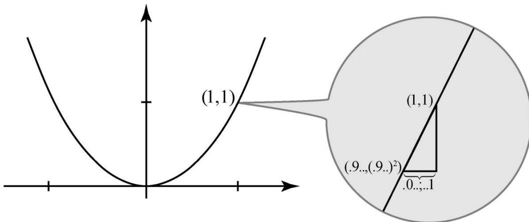
FIGURE 10. Enlargement of an infinitesimal segment of a parabola as calculation of the slope  $f'(1)$  for  $f(x) = x^2$ .
