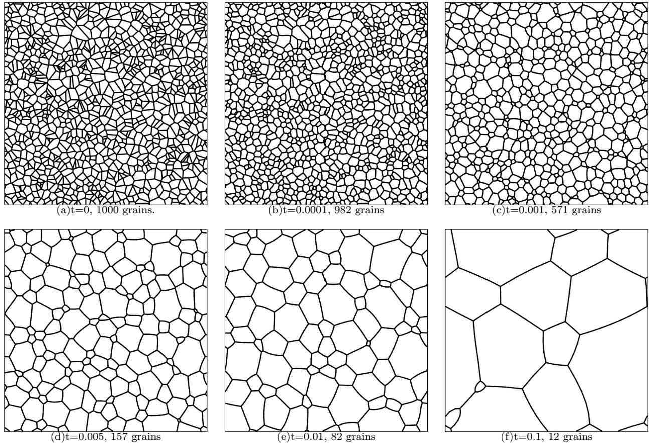
FIG. 7. Temporal evolution of a microstructure based upon the proposed method for  $M\gamma L^2 = 1$ . This microstructure was initialized as a Voronoi tessellation of the unit square into 1000 grains.
