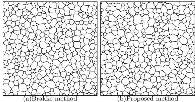
FIG. 8. Microstructures evolved from a single Voronoi tessellation of 1000 grains after half of the grains have been consumed, using (a) the Brakke method and (b) the proposed method.
