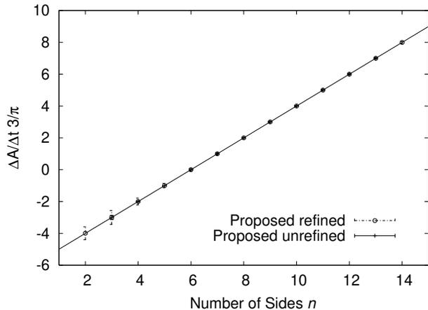
FIG. 12. Validation of the von Neumann-Mullins relation from data obtained using the proposed simulation method with both a refined and an unrefined discretization;  $M\gamma$  is set to 1. The von Neumann-Mullins relation predicts that the points will fall on the line shown. The points here represent data averaged over all grains and time steps in simulations that began with 10,000 grains and ended with 5000. The error bars here show the standard deviations magnified by a factor of 100.
